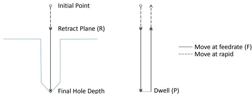
Figure 891-1: Motion of tool point for G89.1 cycle
