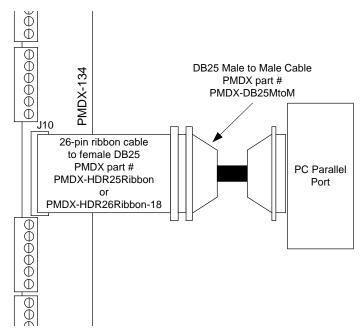
Figure 3 - PMDX-134 connected to PC parallel port
