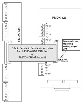
Figure 2 - PMDX-134 connected to a PMDX-126
