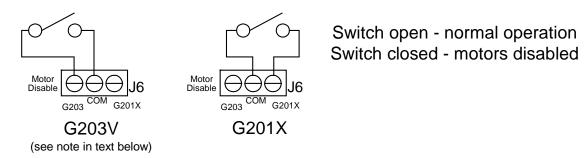
Figure 5 - Motor Disable Sample Connections
