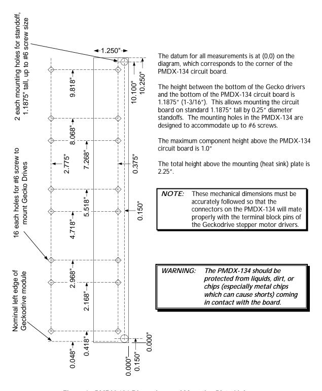
Figure 6 - PMDX-134 Dimensions and Mounting Plate Holes
