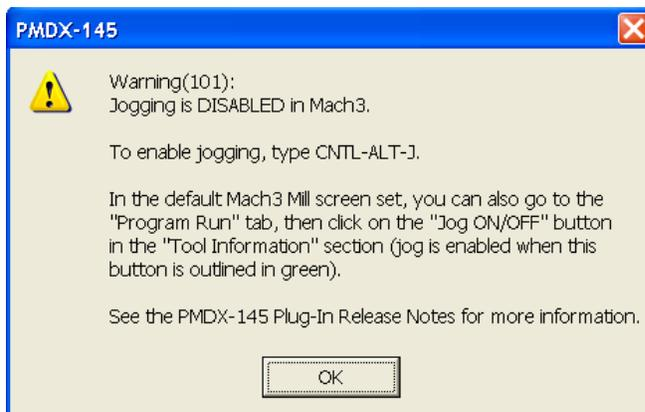
Mach3 allows you to disable jogging so that someone accidentally touching the jog keys on the keyboard will not cause the machine to move. If you are using the default Mach3 mill screen set (see below), then you can see the jogging status and turn jogging on and off with the “Jog ON/OFF” button (in the “Tool Information” section). The button has a green outline when jogging is enabled.
